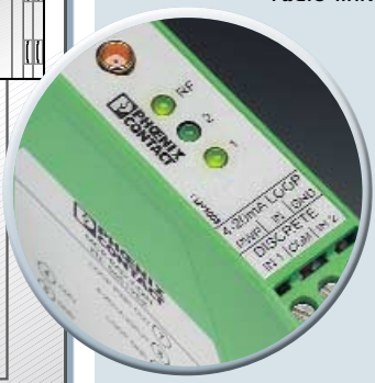
The receiver generates the three sensor signals and the radio link signal. The state of the radio signal can be diagnosed using the radio link signal.
